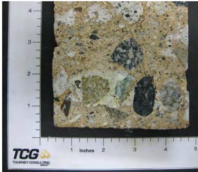
Figure 12 – Example of white crystalline deposits exuded on the surface of core P19-20S
