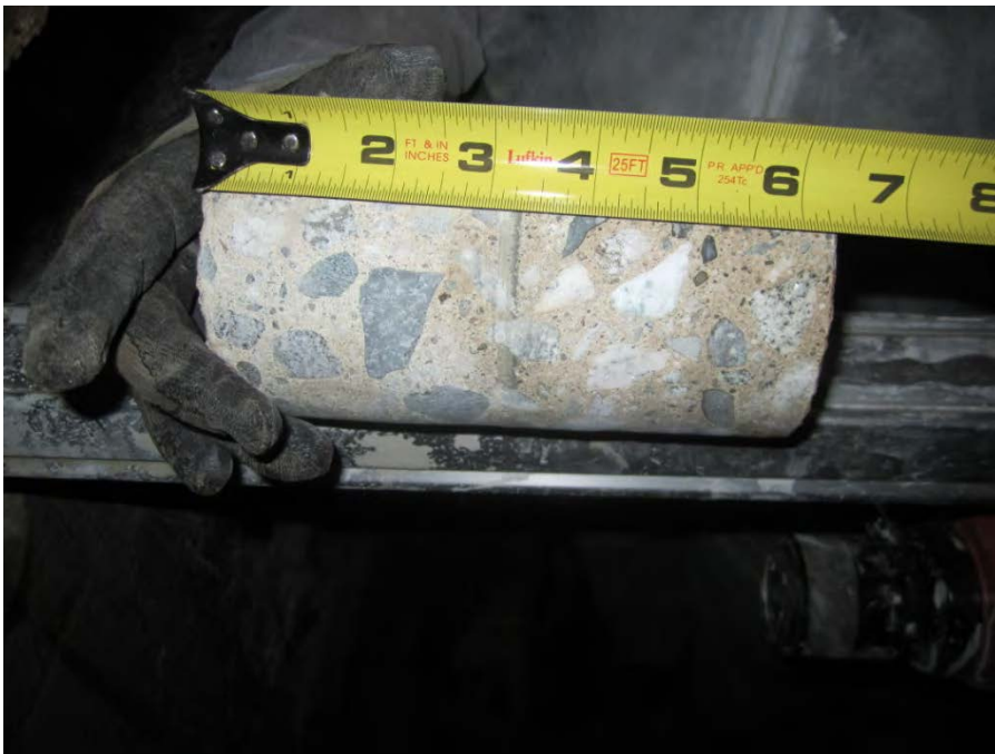
Picture #72- Core CS19-20-S taken to full depth approximately 6-1/4"
