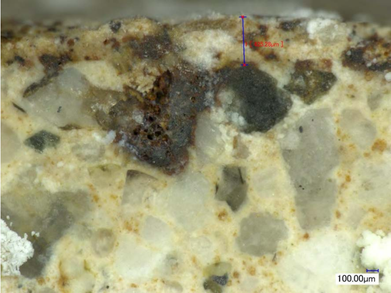
Figure 2 – Brown cement-based coating on the surface of the core
