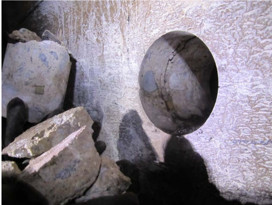
Picture #69- Visible delaminated layer in core hole Petro19-20-S
