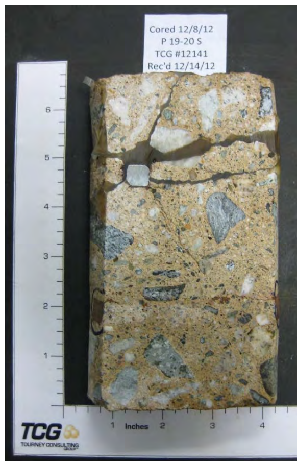
Figure 18 – Core P19-20S after staining with phenolphthalein showing lack of pink staining through the entire section of the core
