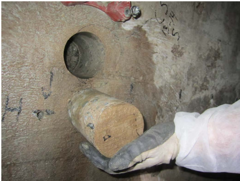
Picture #74- Compressive Strength Core CS13-14S
