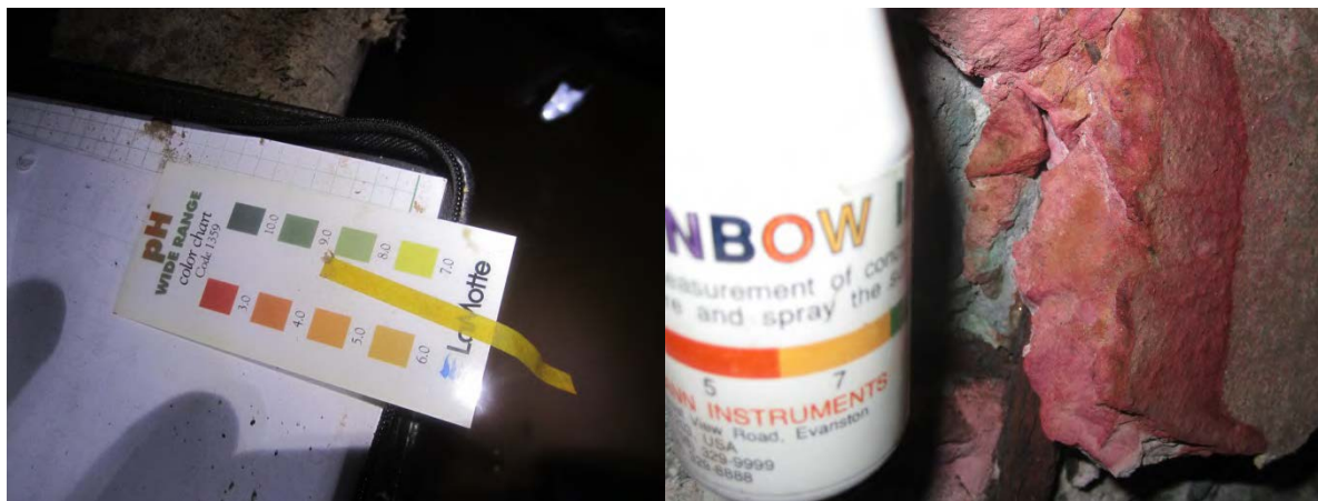
Figure 6 - pH testing of concrete
