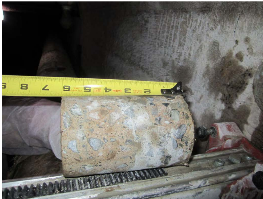
Picture #76- Full depth core CS13-14N approximately 6" thick
