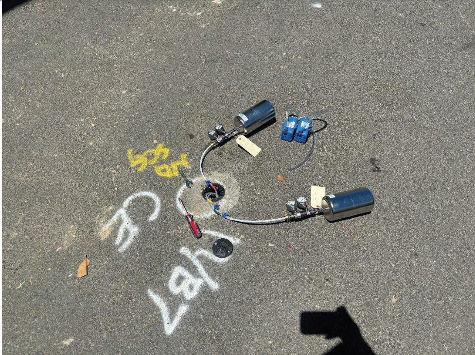
PHOTO 27: View of soil vapor sampling at boring M/B-7.
