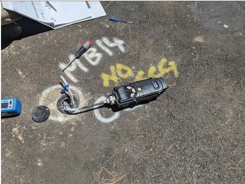
PHOTO 24: View of PID readings at boring M/B-14.
