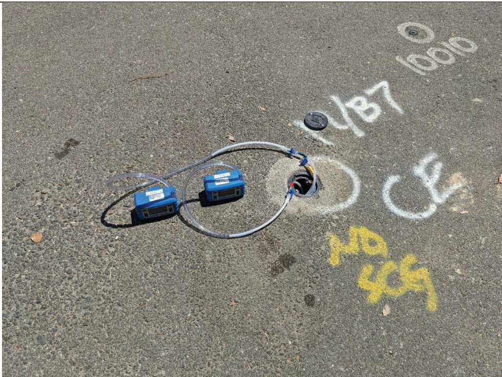
PHOTO 26: View of purging soil vapor probes at boring B-7.
